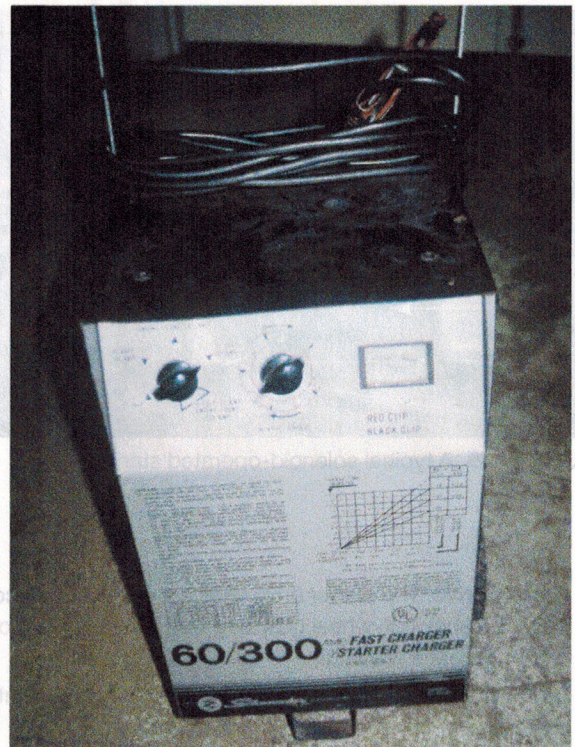
FIGURE 23-8 A typical industrial battery charger. Be sure that the ignition switch is in the off position before connecting any battery charger. Connect the cables of the charger to the battery before plugging the charger into the outlet. This helps prevent a voltage spike and spark that could occur if the charger happened to be accidentally left on. Always follow the battery charger manufacturer's instructions.
