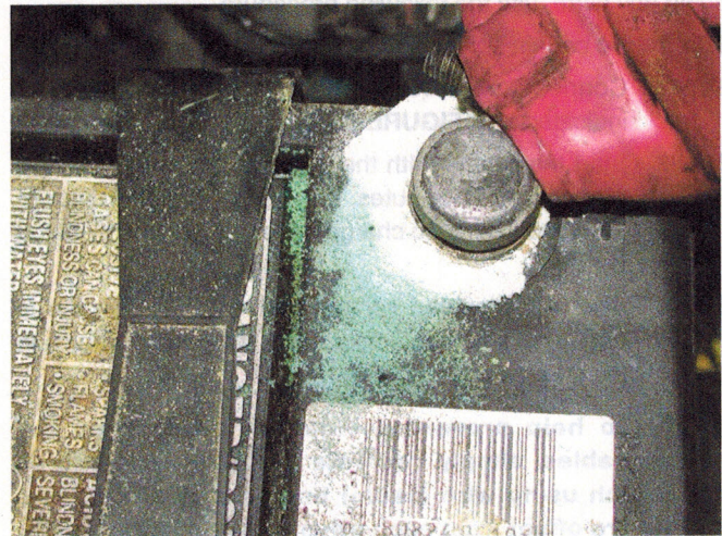
FIGURE 23-11 All battery cables and connections have to be clean and tight for the starter to be able to operate correctly.
