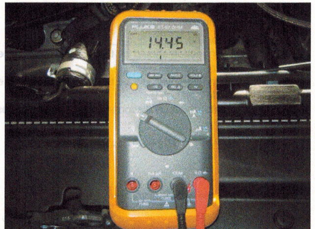
FIGURE 23-13 The digital multimeter should be set to read DC volts, with the red lead connected to the positive (+) battery terminal and the black meter lead connected to the negative (-) battery terminal.
