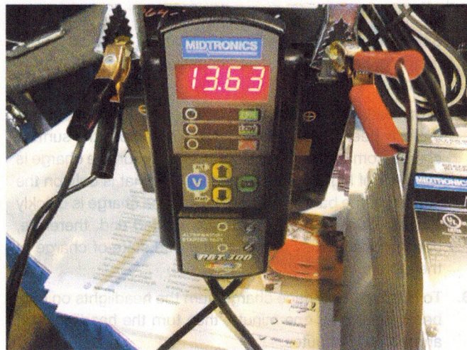
FIGURE 23-6 A conductance tester is very easy to use and has proved to accurately determine battery condition if the connections are properly made. Follow the instructions on the display exactly for best results.
