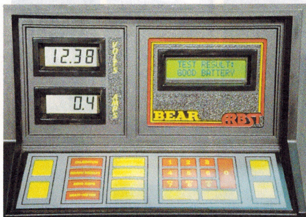
FIGURE 23-5 An alternator regulator battery starter tester (ARBST) automatically loads the battery with a fixed load for 15 seconds to remove the surface charge, then removes the load for 30 seconds to allow the battery to recover, and then reapplies the load for another 15 seconds. The results of the test are then displayed.
