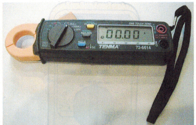
FIGURE 22-12 A typical mini clamp-on-type digital multimeter. This meter is capable of measuring alternating current (AC) and direct current (DC) without requiring that the circuit be disconnected to install the meter in series. The jaws are simply placed over the wire and current flow through the circuit is displayed.
