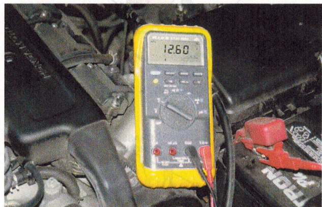
FIGURE 22-5 Typical digital multimeter (DMM) set to read DC volts.
